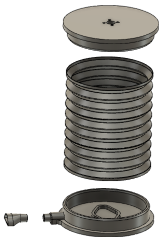
Figure 2. CAD model of bellow module.
